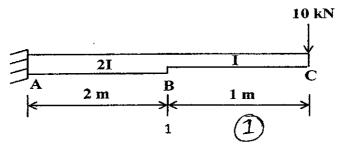
S.Y.B.Tech. (civil) SemIV Structural Analysis-I - Dt - 06 loll 16. Q.2 (b) Find the slope at B and vertical deflection at D for the beam supported and (12) loaded as shown in figure below. Use conjugate beam method only.
